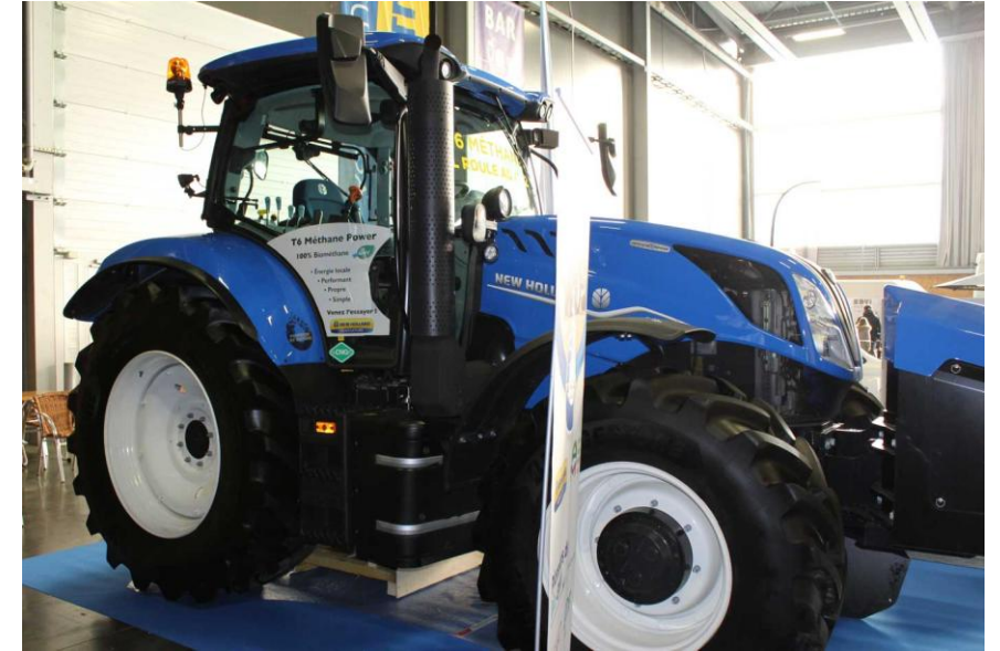
• New Holland T6 180 Methane Power
