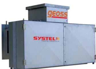
**Major innovation:** First progressive heating system incorporating flame-locked burner (15-85 kW without extinguishing at 10 m/s wind speed) and intelligent dual ventilation (combustion air + dilution with 0-100% recycling)
