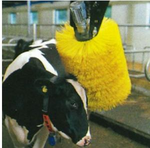
**Major innovation:** First cow brush combining dual motion (rotation + pendulum oscillation) activated by simple contact from the animal, along with intelligent mapping via electronic card and dual ball contact system
