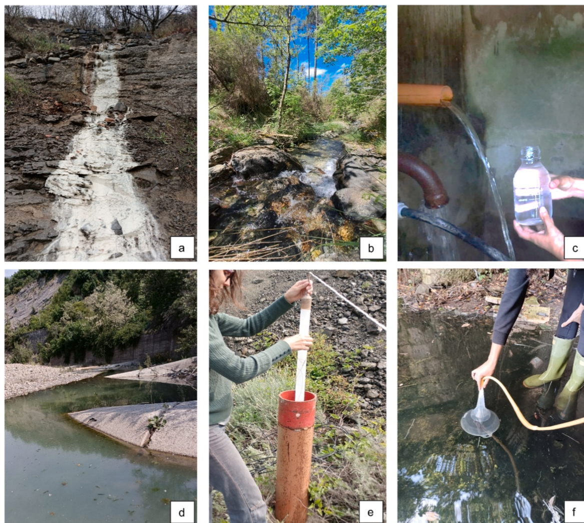
Fig. 2. Photographs illustrating various sampling methods and spring water types: a) natural spring water, exhibiting a white track in the wall (Bobbio1); b) hyperalkaline spring water coming out of ophiolitic rocks (Issel), c) tapped spring water sampling (Sagos3); d) bubbling spring water forming a pond close to the Trebbia River's margin (Bobbio4); e) borehole water sampling (Mzir), and f) bubbling spring gas sampling (Bobbio3).
