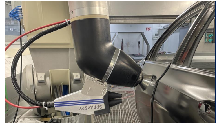
SpraySpy® attached to bell atomizer.
