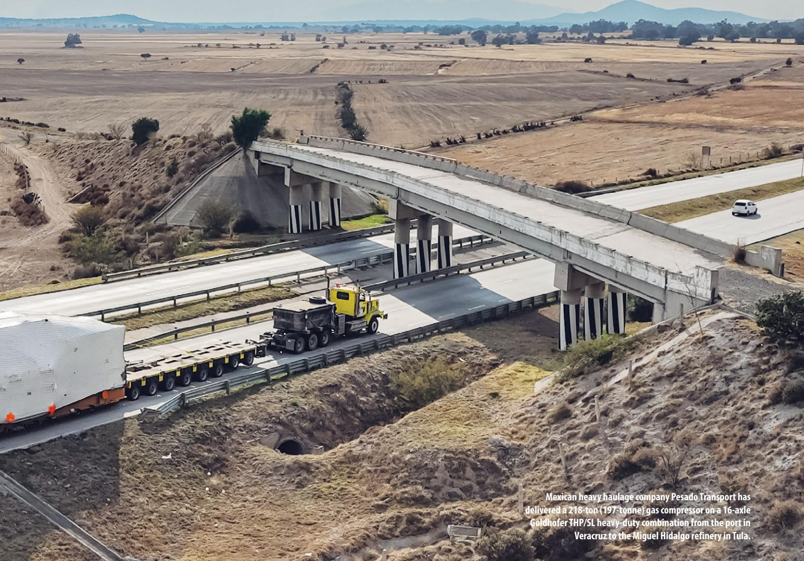
**Mexican heavy haulage company Pesado Transport has delivered a 218-ton (197-tonne) gas compressor on a 16-axle Goldhofer THP/SL heavy-duty combination from the port in Veracruz to the Miguel Hidalgo refinery in Tula.**
