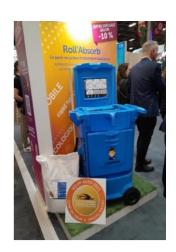
The mobile workshop cleaning trolley is designed as an all-in-one. It stores waste, and dispenses and recycles the Chimirec LIQ-LOCK absorbent agent which has superior absorbency capacity thanks to its ligno-cellulosic fibre fine honeycomb structure. The soiled product is isolated using an internal sieve, and the reusable product is returned to the cleaning agent stock.
